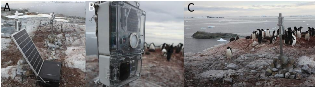
Figure 4: Deploying the first satellite linked camera on the Yalour Islands, Antarctic Peninsula. A) shows the camera setup with power solution. B) Close up of the camera and node. C) View of camera with the view of the penguin colony.
